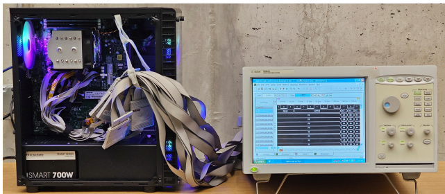
Figure 1: Our memory interposition setup, with target machine (left) and logic analyzer (right). Notice the gray wires from the DIMM interposer (middle).
